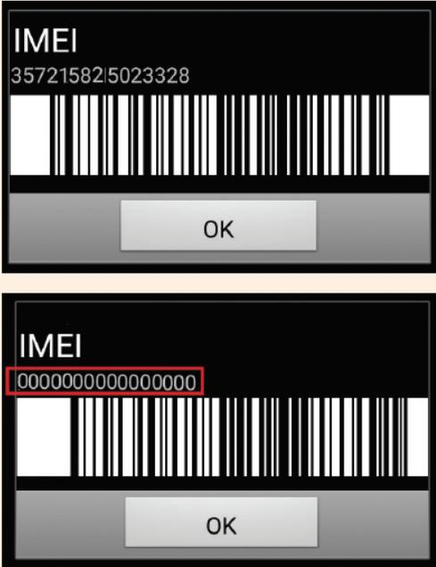
At the top, a genuine IMEI number found on a sticker inside a feature phone. Inputting the discovery code **\*#06#** will show that the original IMEI number has been replaced with a set of zeros (on the bottom). These changes hide the phone's true identity.<sup>115</sup>
